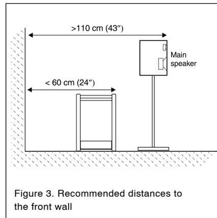
Figure 3. Recommended distances to the front wall
