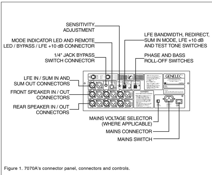
Figure 1. 7070A's connector panel, connectors and controls.
