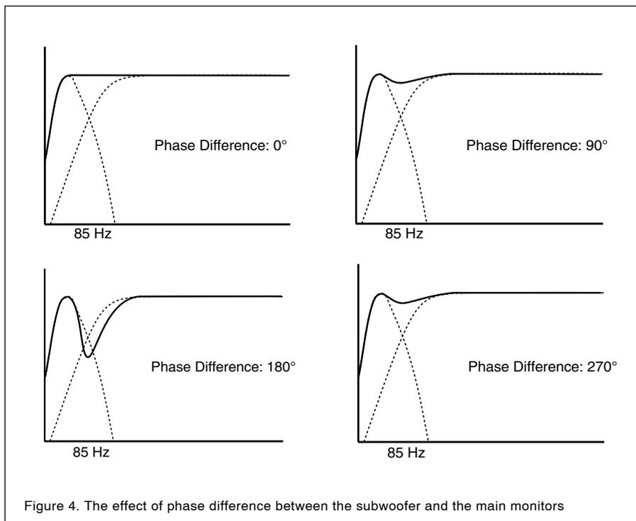
Figure 4. The effect of phase difference between the subwoofer and the main monitors
