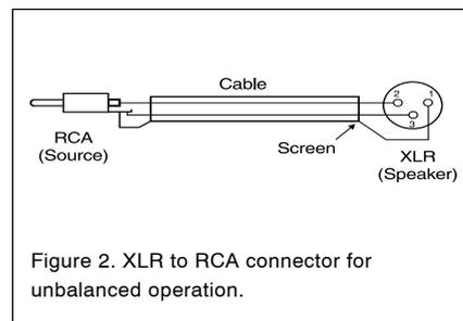
Figure 2. XLR to RCA connector for unbalanced operation.
